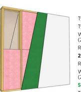
Type X Drywall 15.9 mm (5/8") Type X Drywall 15.9 mm (5/8") Wood studs 50.9 mm x 101.6 mm (2" x 4") at 610 mm (24") c.c. R-12 Batt Insulation
