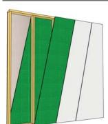
Type X Drywall 15.9 mm (5/8") **SONOpan** 19 mm (3/4") Wood studs 50.9 mm x 139.7 mm
