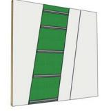
50.9 mm x 101.6 mm (2" x 4") aux 406 mm (16") c.c. R-12 Batt Insulation Drywall Adding:
