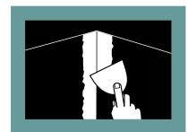
OUTSIDE CORNERS Apply a band of joint compound 100mm (4") wide and 6mm (1/4") thick to each side of the corner.
