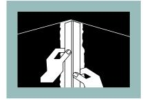
Cut corner bead to length required and position over the joint compound allow 1/2" at bottom for expansion and contraction of framing members.
