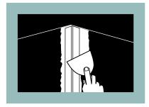
Embed the corner bead firmly into the compound. Using a small finishing knife, wipe the excess compound from under the paper to eliminate all air bubbles. Allow to dry. (Be careful not to remove all compound)
