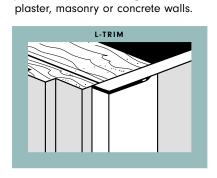
L-Trim is used to trim wallboard where it abuts with untrimmed door and window jambs, suspended ceilings, beams and
