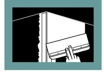
Using a large finishing knife, apply compound in a band about 200mm (8") wide from the nose of the bead beyond the paper edge.
